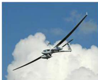
Figure. Motor glider Antares DLR-H2 with two pods for hydrogen tanks and fuel cell system; flight profile on November 21 st , 2009.
