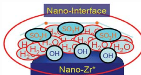
Figure 2. The schematic illustration of a nano interface between s-ZrO 2 & SPES.
